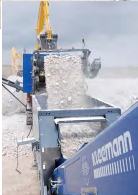
Hoskins Gypsum uses Kleemann crushers and screens at Hoskins Quarry. The company also owns several Komatsu machines, including a PC350LC-8 excavator, shown here loading the crusher.
