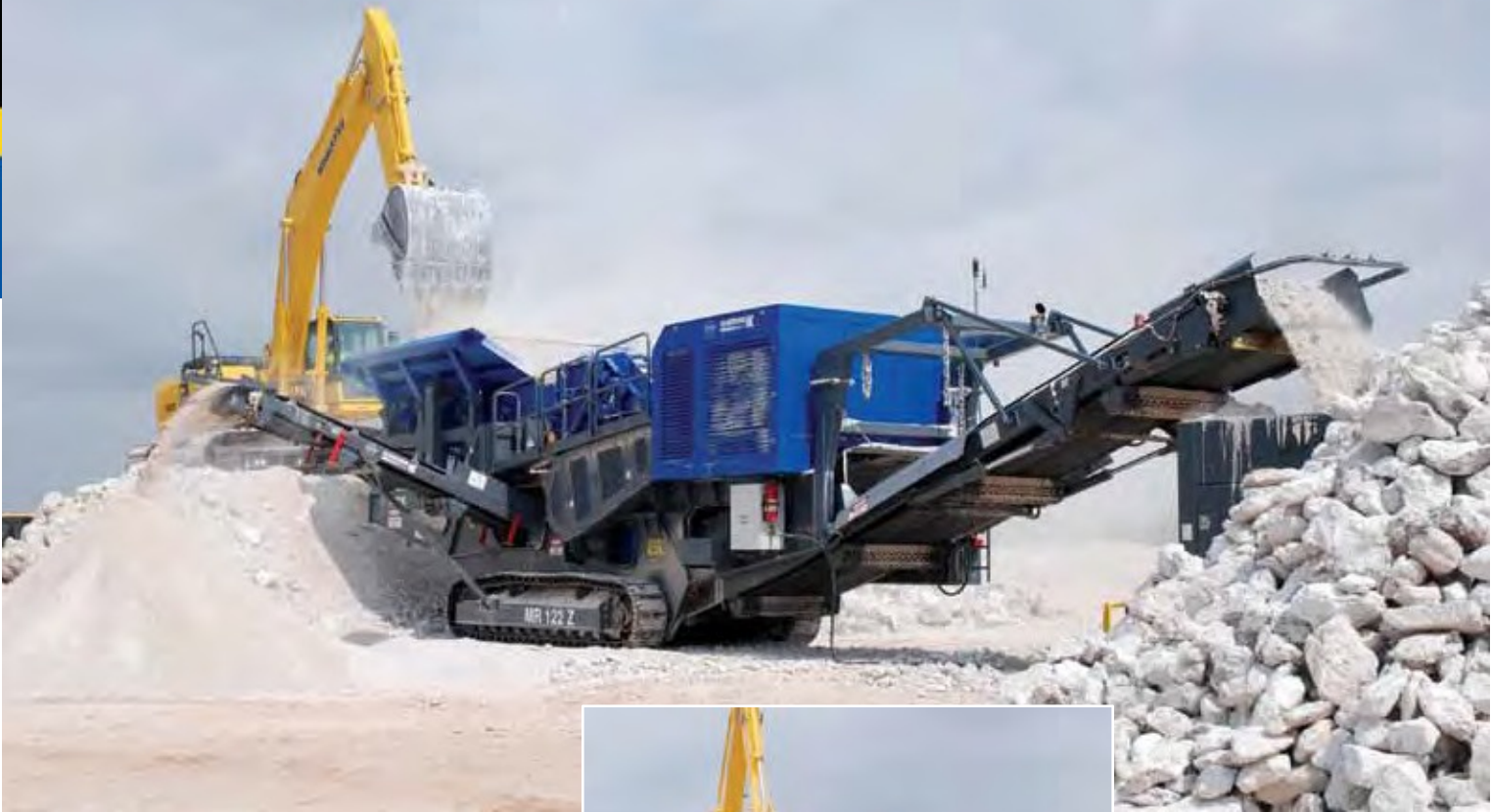
Hoskins Gypsum uses Kleemann crushers and screens at Hoskins Quarry. The company also owns several Komatsu machines, including a PC350LC-8 excavator, shown here loading the crusher.
